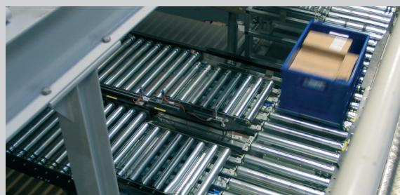
achieved. The system's acceleration and braking performance is also enhanced. This increases the positioning accuracy and thus safety, as contact between sensitive goods on the roller conveyor is therefore be avoided. So it's no surprise that roller conveyor system manufacturers also recommend ContiTech belts.
